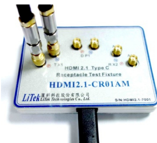
Fig 2: HDMI2.1-CR01AM plugged into Host Device after Type C to TypeC cable assembly
